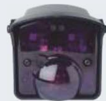
Radar / presence detector Comfort Radar movement and presence detection with infrared detection, fast and targeted automatic door opening, reliable advance protection, up to a height of max. 6 m, in areas with high levels of humidity and in outside areas, only the radar function is available, housing: protection category IP 65
