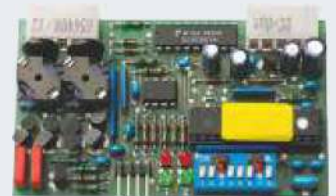
Induction loop detector 1 or 2-channel plug-in print suitable for two separate induction loops, supplied without loop cable
