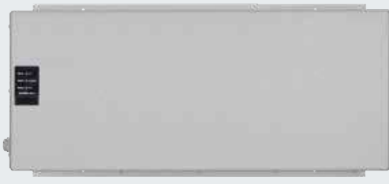
UPS system For bridging power failures of up to 4 hours, safety devices, warning lights, etc., remain functional, LED status display, automatic battery test, surge filter, dimensions: 560 × 235 × 260 mm (W × H × D), protection category: IP 20
